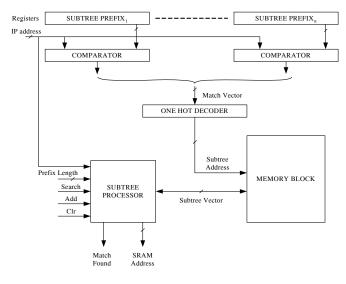
Fig. 3. Architecture of a level module
